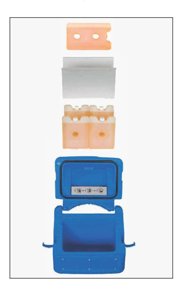
MT4-ET-32, ambient temperature +43°C, Dummy temperature -40°C Load 2xGFP-D, 1x600ml ET-32, 4x300ml ET-32
