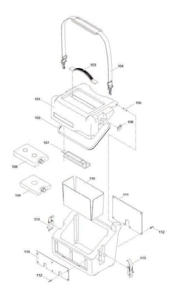
Thanks to the use of eutectic thermal energy storage elements, the range of use can be significantly extended. Here, specially adapted thermal energy stores in two sizes can now be used for different temperature ranges. The nominal volumes are 600 ml and 300 ml.
